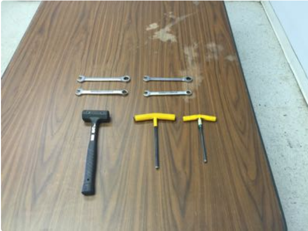
1. Tools needed: 2 - 9/16 wrenches, 2 - 1/2 wrenches, 1 - 1/4 allen wrench, 1 - 5/16 allen wrench, 1 - hammer
