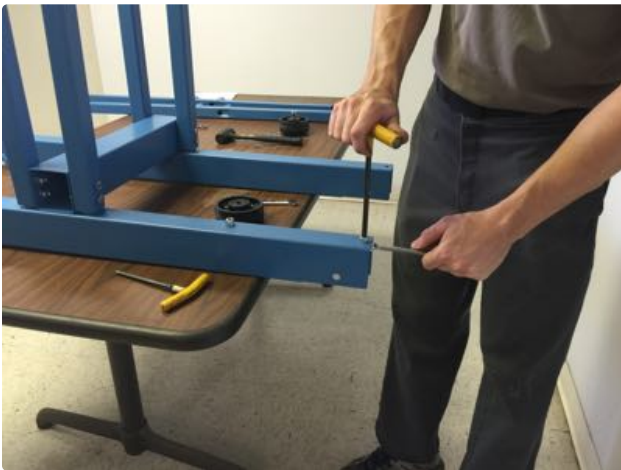
8. Mount and tighten the 3/8-16 x 1/2 socket head bolt and nut on to the leg.
