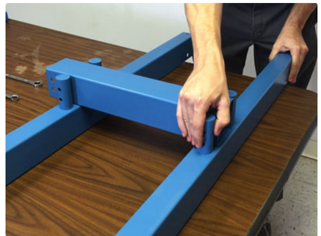
5. Place the legs on a flat surface and space them apart with the bottom cross member (the one without the label) so that the holes in the cross member align with the holes on the posts.
