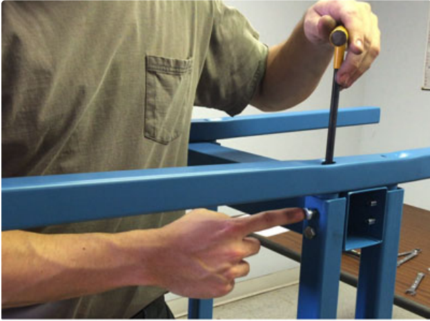
13. You may have to loosen the bolts that hold the post in place in order to insert the bolts into the cross member.
