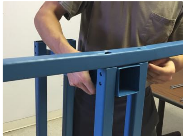
11. Position the top cross member (the one with the label) between the columns, align the holes using the 3-8/16 x 2 hex head bolts.
