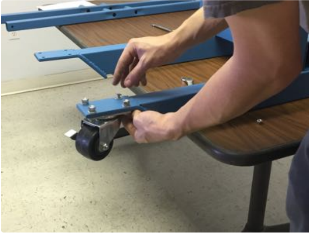
7. Mount the casters to one end of the leg using the 5/16 -18 x 1 hex head bolts, washers, lock washers and nuts. Tighten the bolts.
