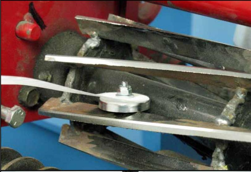
Keep tension on the pi tape as you rotate the reel and wrap the pi tape around the reel.
