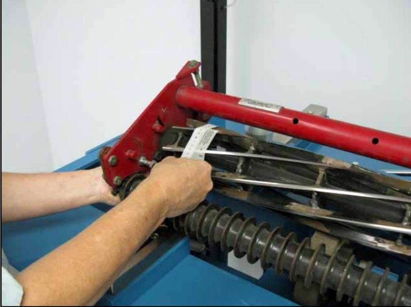
Make sure that you wrap it in a straight line so that the end of the tape lines up with the beginning of the tape and that the edge of the tape lines up with the vernier line.
